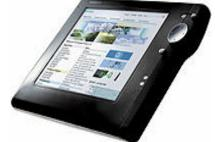
As a small example of the 'carry-with-you' kind of computing that depends on wireless connection, German manufacturer Siemens has recently unveiled a device it calls the Gigaset 4600 SIMpad<sup>10</sup> that allows you to 'carry the Web' around. It's one of several 'Web pads' either in development or coming to market now. When turned on you have almost instant access to the Web. It runs on Windows CE operating system and Internet Explorer, and weighs about two pounds.
