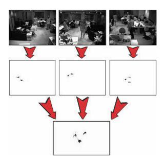
A person-tracking system uses three camera modules, each consisting of stereo camera and a computer, that are arranged to view an entire room and continually estimate 3D-point clouds of the objects in the room. The system clusters foreground points into blobs that represent people, from which it can extract features such as a person's location and posture.
