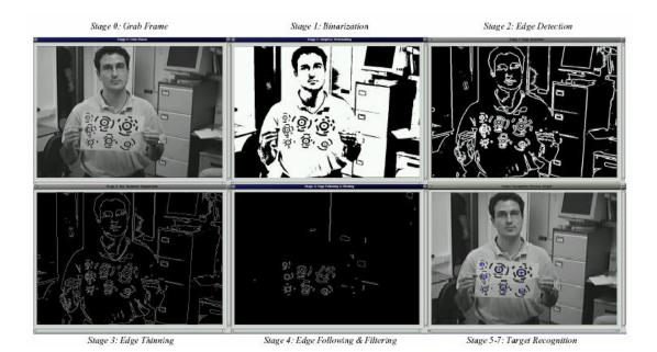
Stages in identifying and locating TRIPtags on a sheet of paper. These could equally be attached to a user's clothing.
